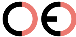
False CE Mark (too far)
